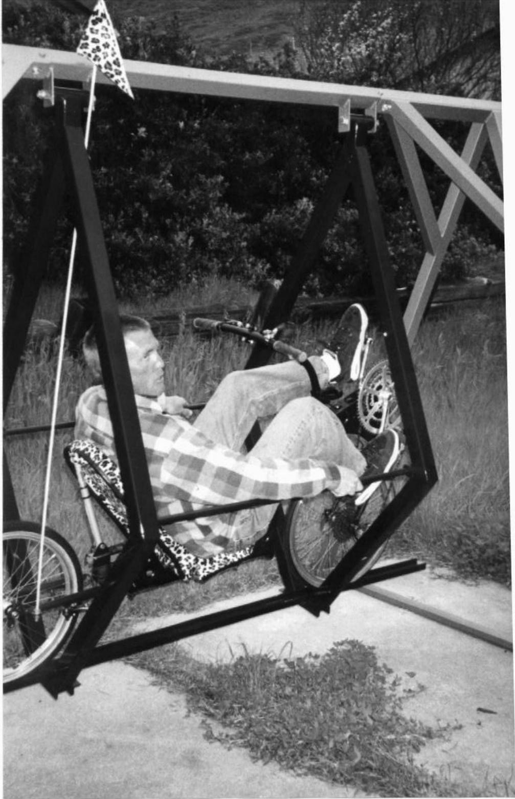
The bike swing is used to determine  $K_x$  for the class project bikes.
